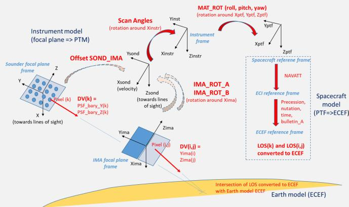
The IASI-NG geometric model is a simplified description of the instrument optics and mechanics aiming at establishing the link between the imager and sounder pixels viewing directions in their respective focal planes and the location of these pixels on the Earth surface (lat/lon coordinates).
