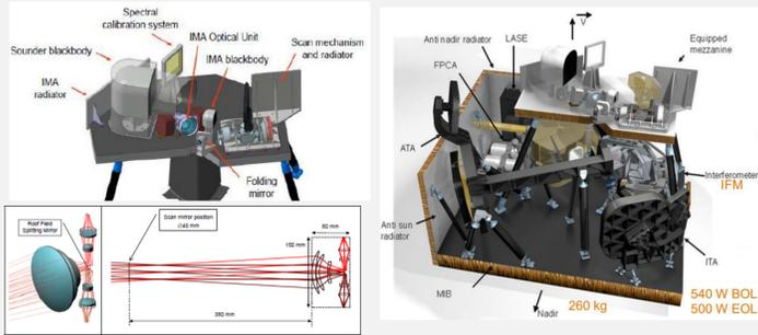
Imager: 2 half-images on different focal planes (2 \* 150x75 pixels) Sounder: 16 sounder pixels on the same plate Common sounder/imager scan mirror
