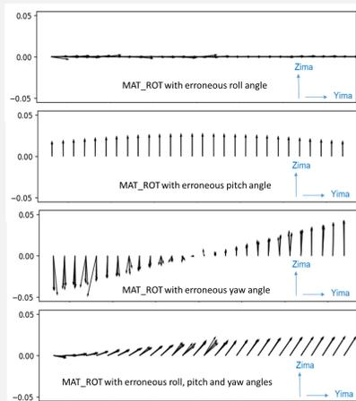
Retrieved offsets in (Y,Z) plane for the 14 IASI-NG scan angles, 2 detectors and 4 BRCs. The offsets are obtained using different configurations of MAT\_ROT combining errors in roll, pitch and yaw Source : outputs of OFFST (COREG) simulations in IRIS
