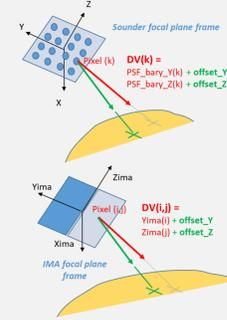
A dynamic adjustment of the sounder and IMA viewing directions is performed at each acquisition using as a reference concomitant METImage L1B radiance in the 10.69 μm channel and L2 CLD products, with a supposedly perfect geolocation.
