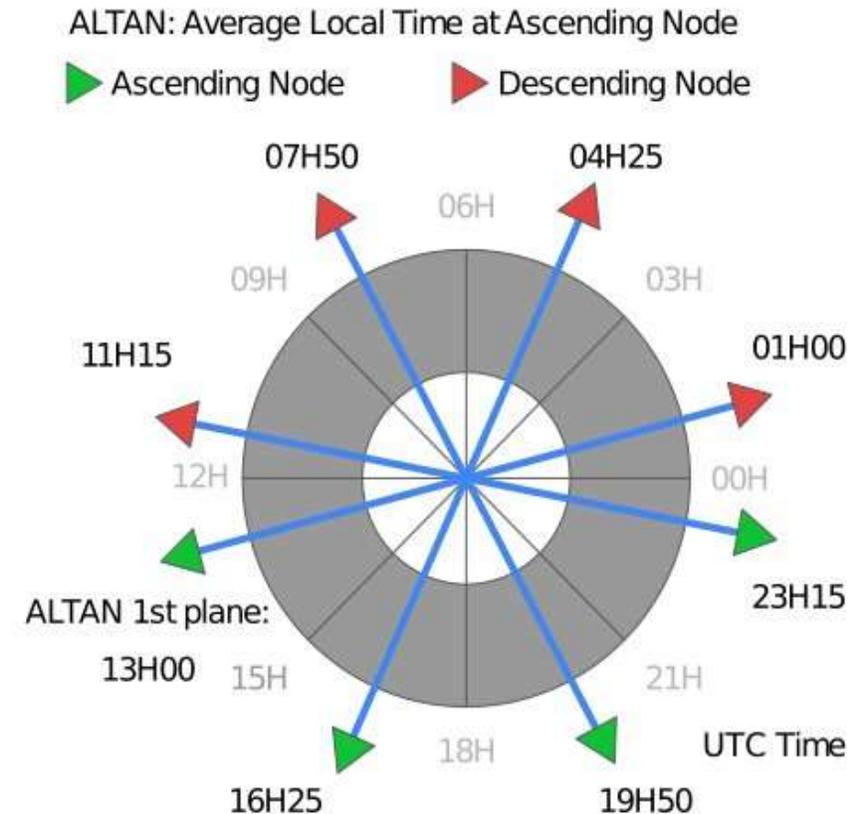
Figure 9. Equatorial cross-sectional plane of the nodes for the reference CMIM constellation : 8 satellites, 4 orbital planes, with a revisit time lower than 3H30 for 95% of cases between 35 and 60 degrees of latitude. Source : CNES (2023)
