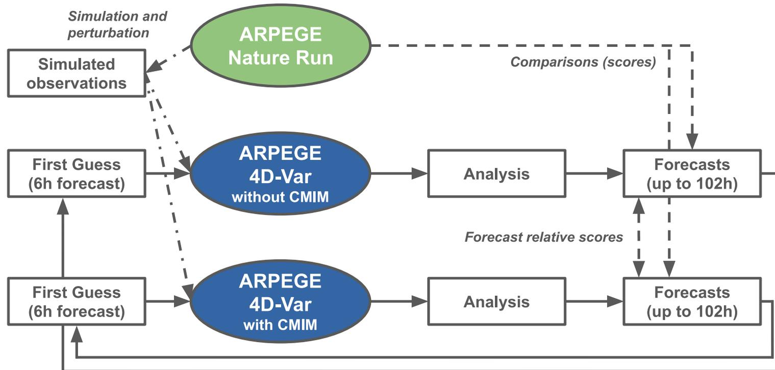
Figure 1. Description of the framework of the OSSE, with and without the CMIM constellation
