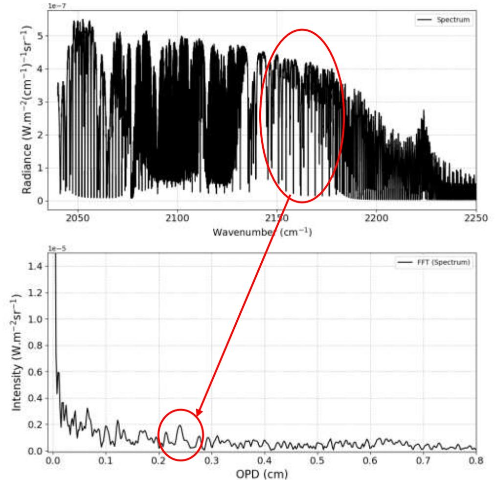
Figure 2 : Spectra and interferogram of the CO signature
