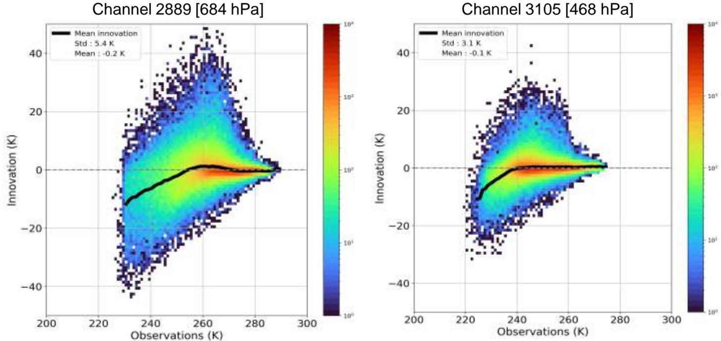
**After applying QC**, the innovation average is close to zero, a good point for moving towards data assimilation.
