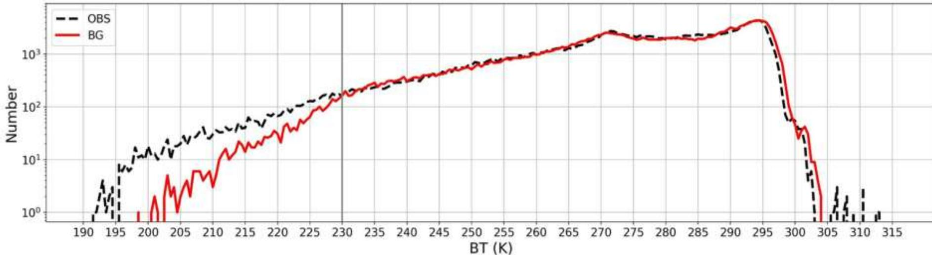
→ The cloud simulation is **correct with respect to observation** except for values below 230 K. Similar to Okamoto et al., 2023 results, we will impose a threshold to only **take into account observations above 230 K (QC)**.
