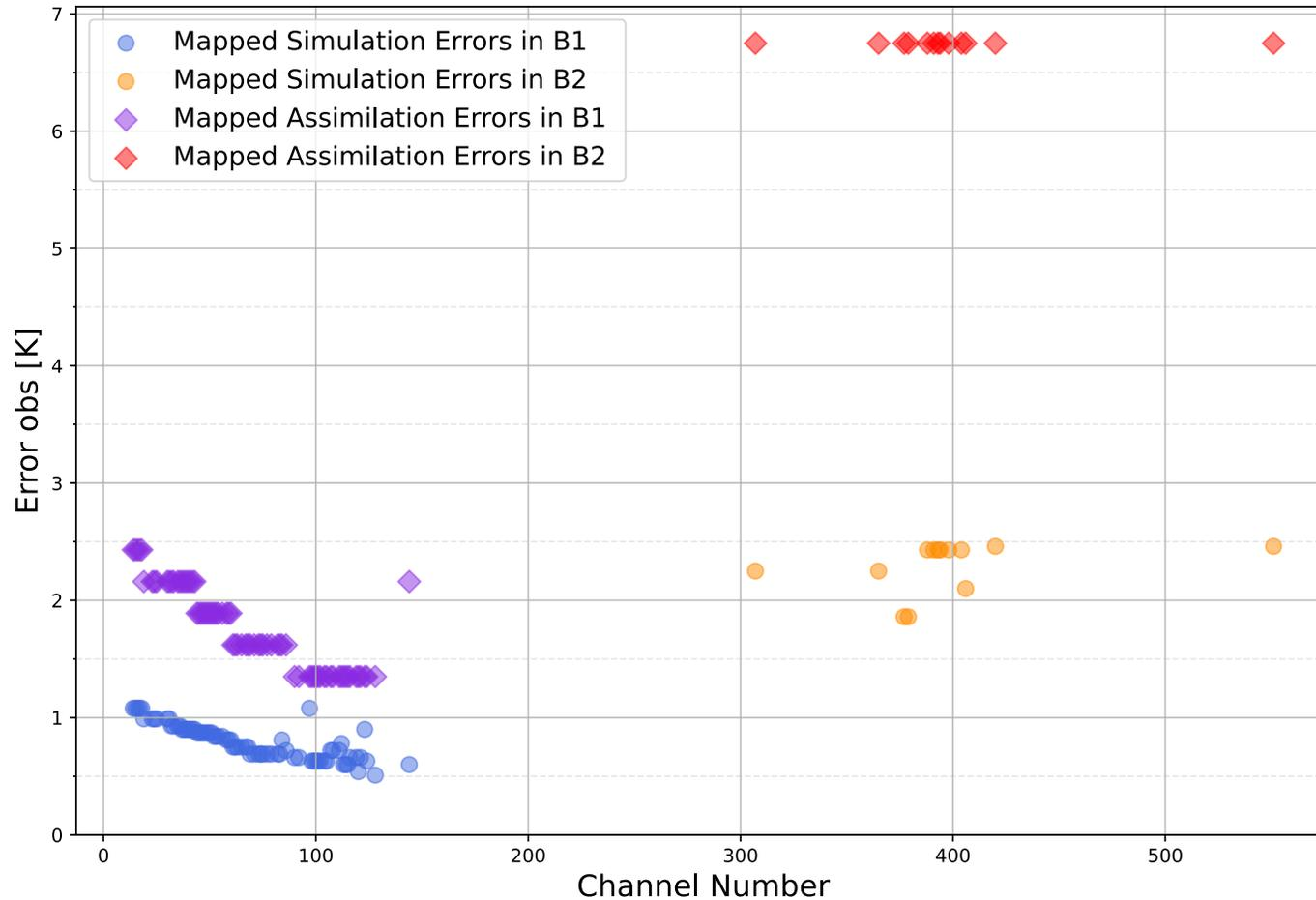
Figure 10. Comparaison of instrumental noise applied to the CMIM-IR reference scenario, mapped from the instrumental noise applied to IASI in Kelvin
