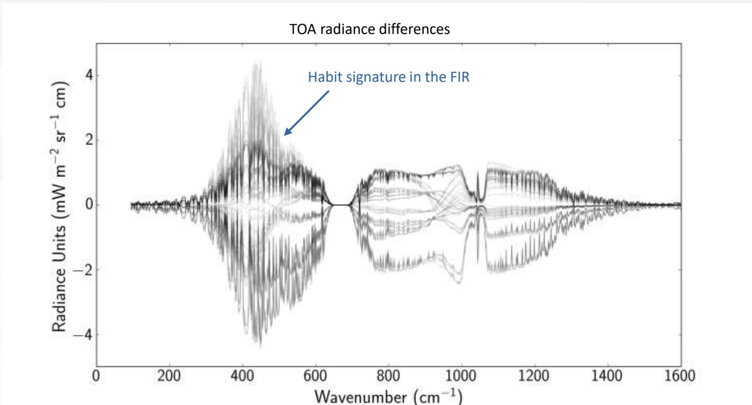
Ice cloud (12 km,  $\tau=3$ ,  $\text{deff} = 60 \mu\text{m}$ ), 9 different ice habits and 3 surface roughnesses
