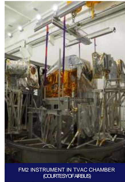
FM2 INSTRUMENT IN TVAC CHAMBER
