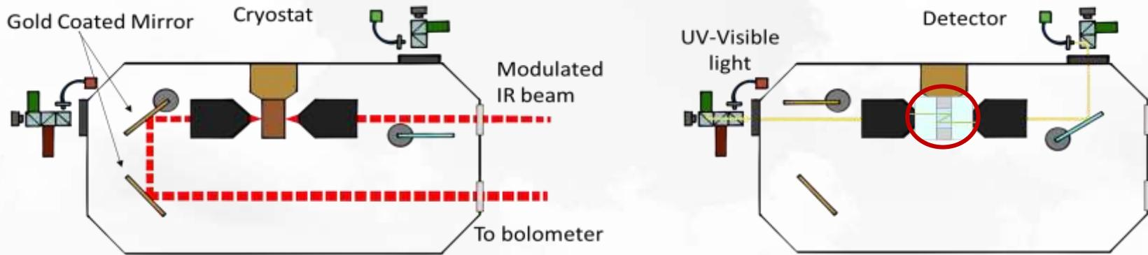
Experimental setup at Synchrotron SOLEIL : transmittance (left) and ice thickness (right) setup
