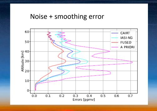
The result of the combination of CAIRT and IASI-NG is characterised by profiles with better spatial resolution and a smaller total (noise + smoothing) error
