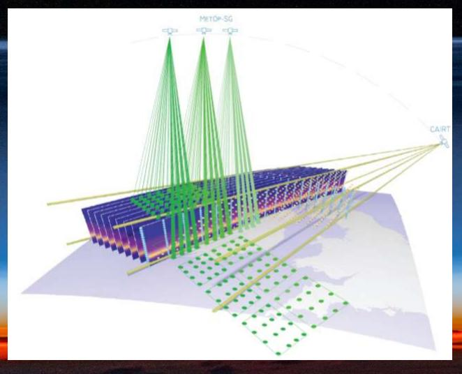
Concurrent limb and nadir (from MetOp-SG-A) viewing allows to extend CAIRT measurements to the lower troposphere, to further constrain the horizontal variability and to exploit the synergy.
