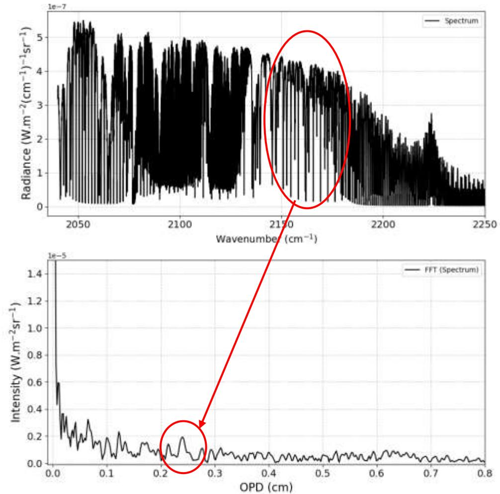
Figure 2 : Spectra and interferogram of the CO signature
